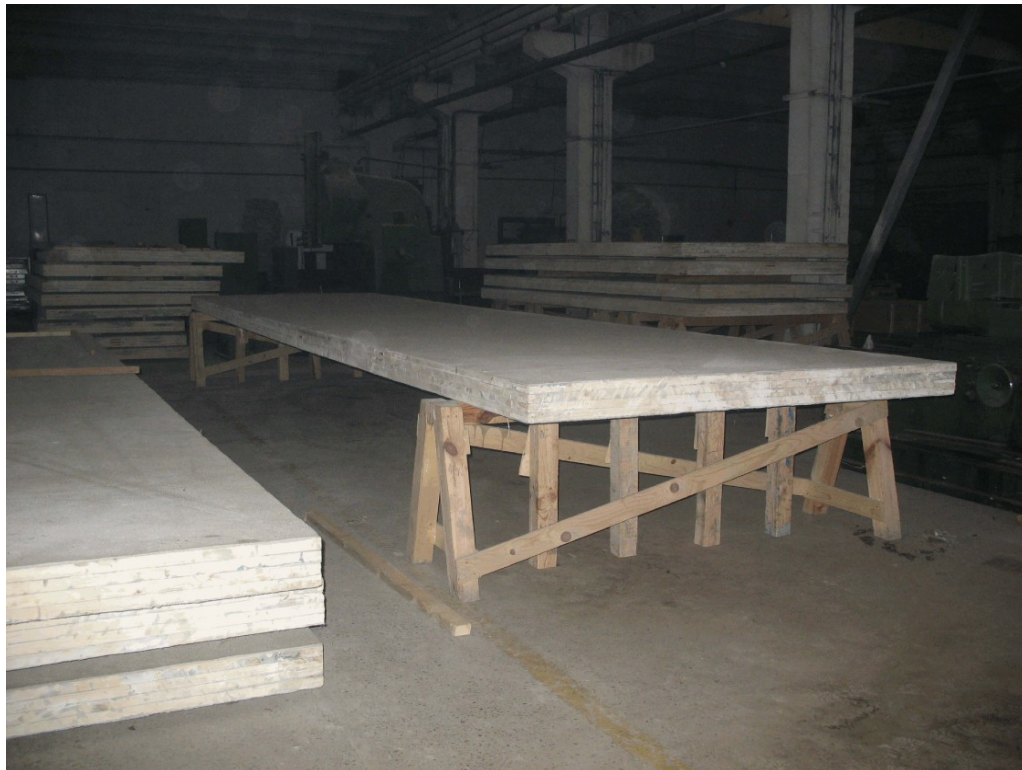
Fig.8 Panel for roof (h = 145 mm ; l = 2.5 m ; L = 10 m)
