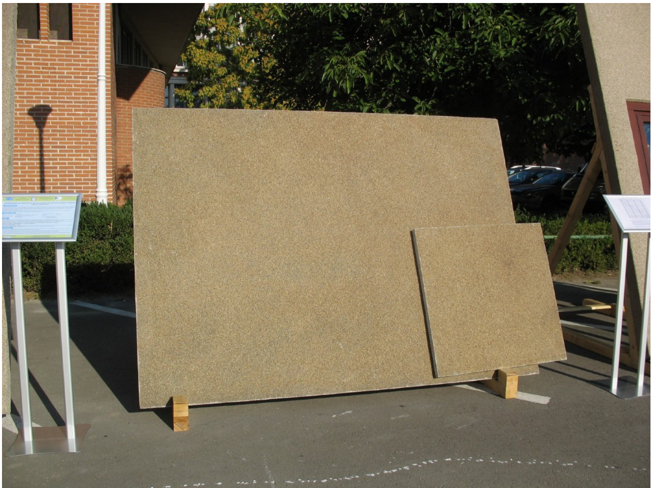
Fig. 6. Panel for thermal insulation (h=50mm, l=1.5m, L= 3 m)
