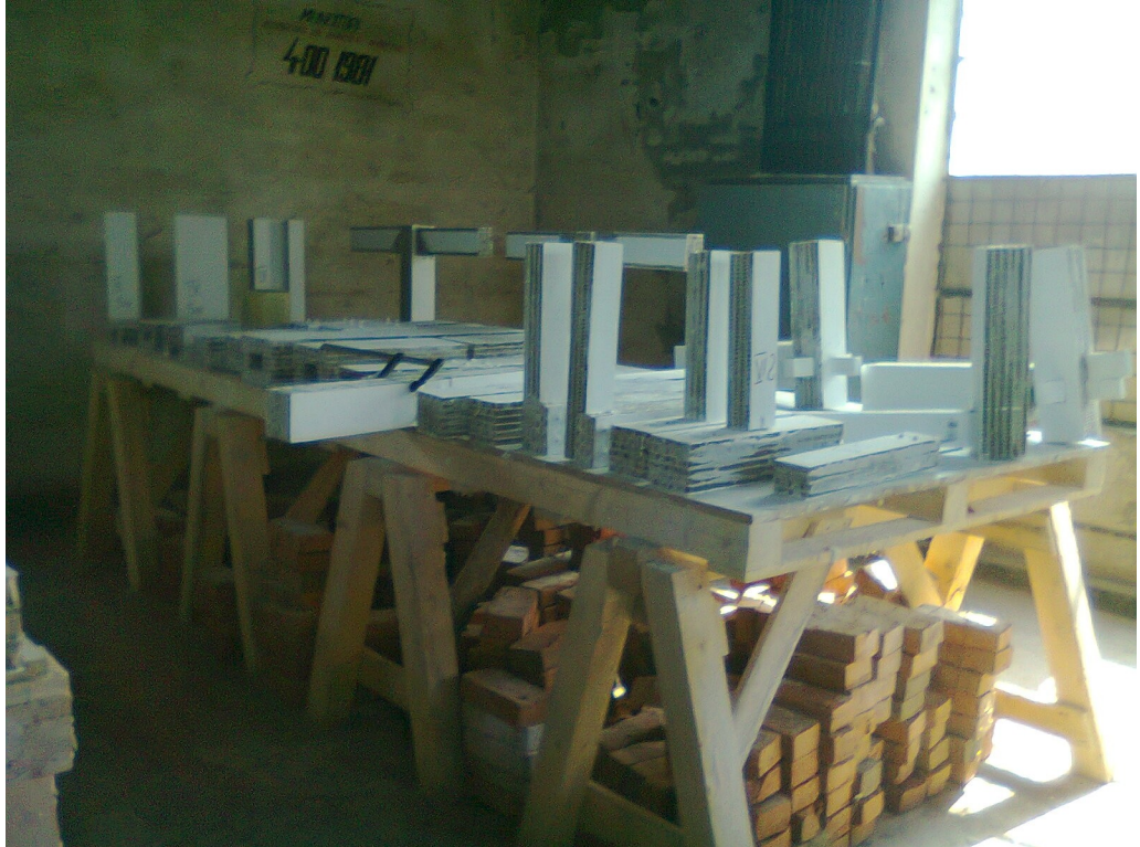
Fig.20. Pillar - crossbeam joining systems (testing samples)
