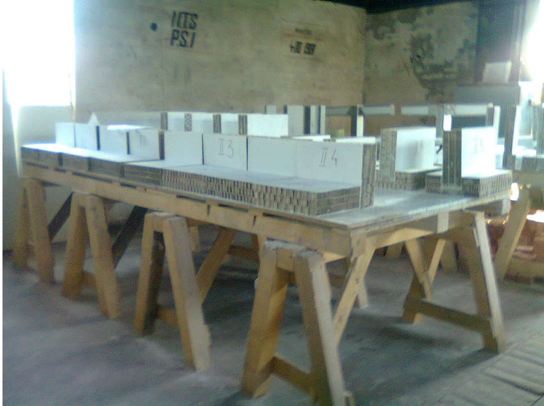
Fig.18. Joining systems for panels at 90° (testing samples)
