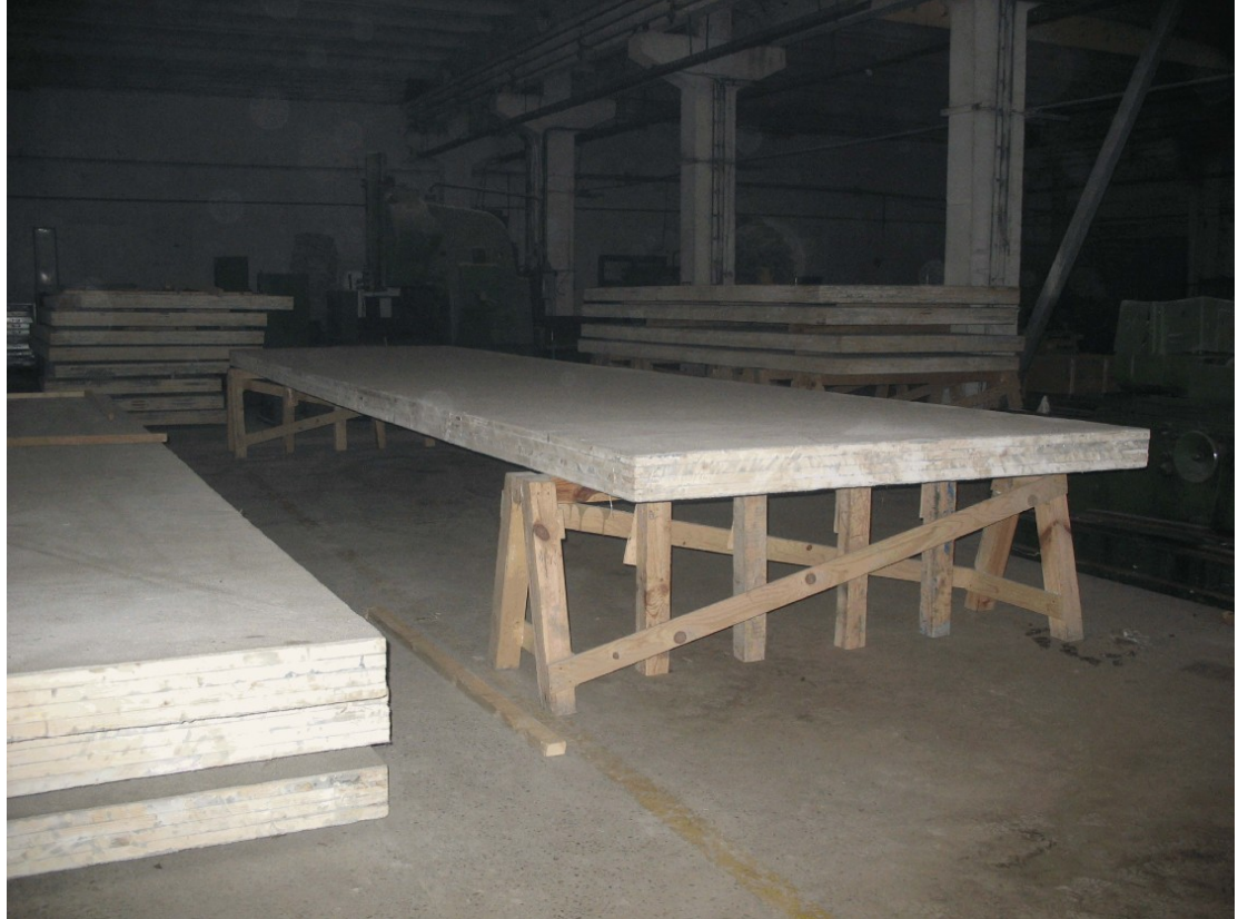
Fig.16. Panel for roof (h = 145 mm ; l = 2,5 m ; L = 10 m)
