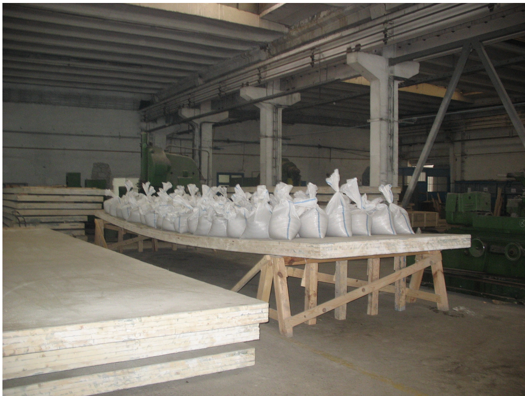
Fig.21. The testing of the roof panel. Weight = 5800 Kg
